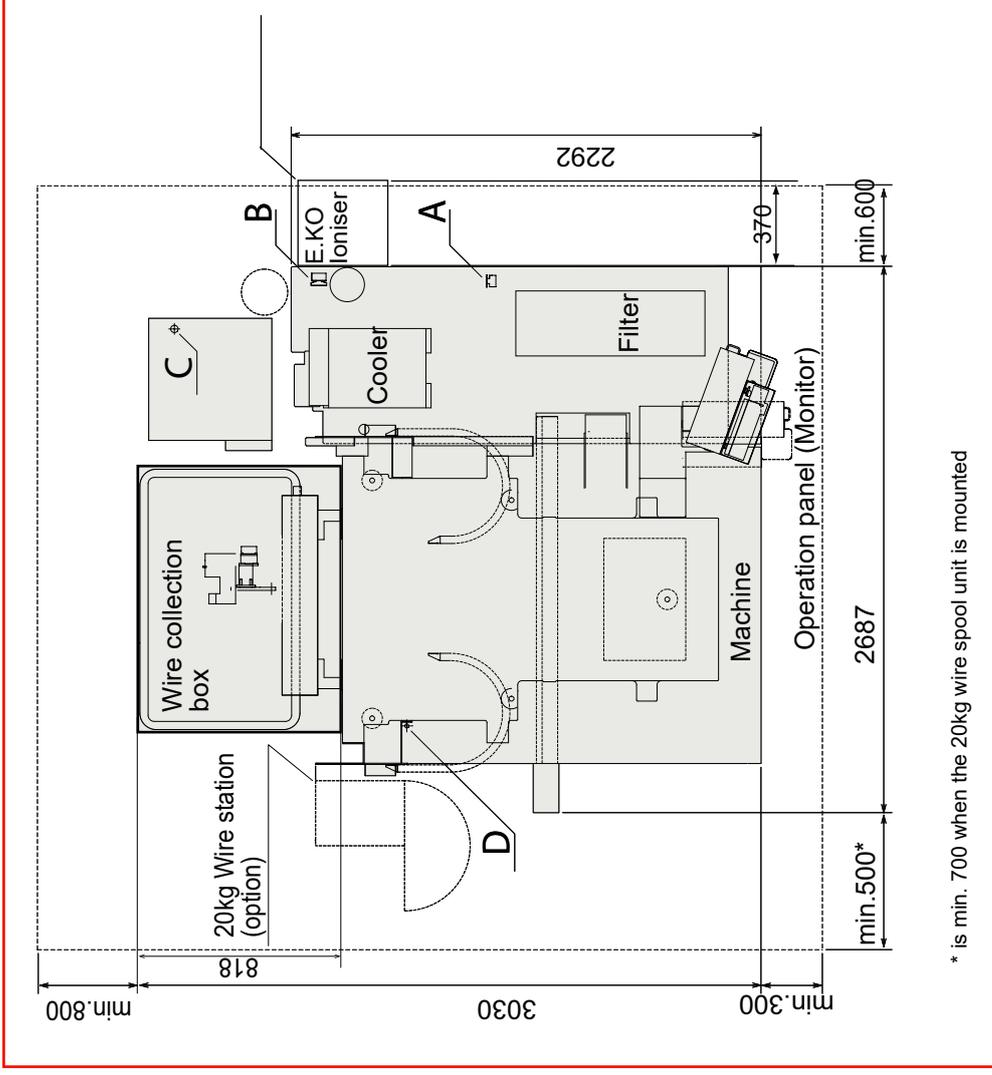
\* is min. 700 when the 20kg wire spool unit is mounted
